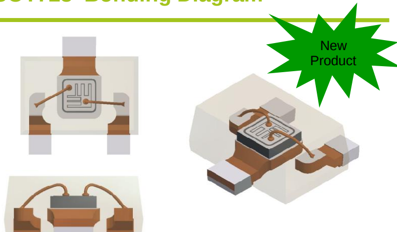
SOT723 Bonding Diagram
