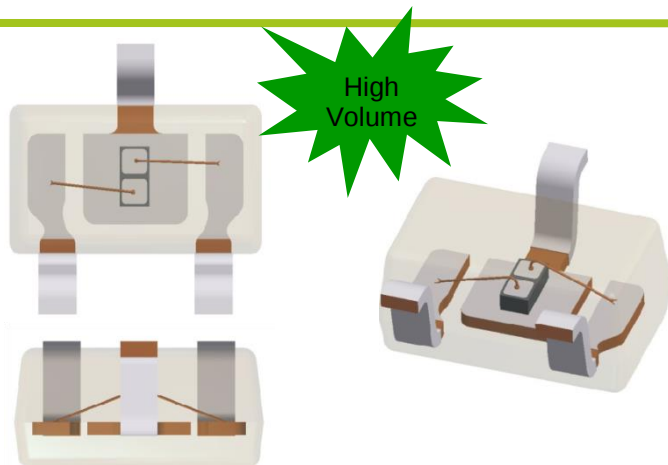
SOT323 Bonding Diagram
