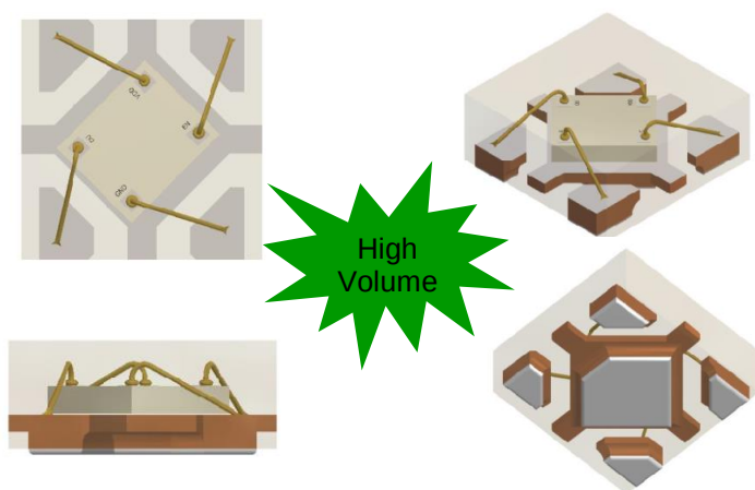
DFN1107-6L Bonding Diagram
