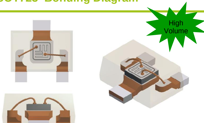
SOT723 Bonding Diagram
