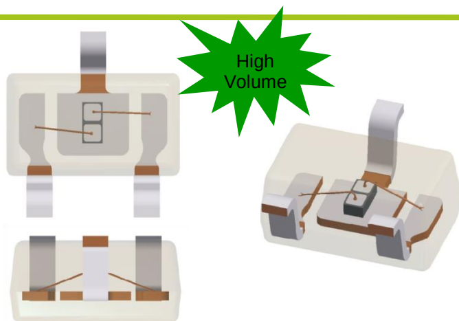
SOT323 Bonding Diagram
